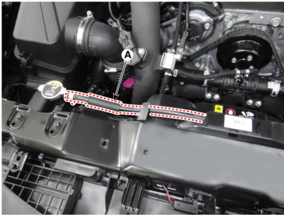
2. Remove the LH front strut bar (A).
