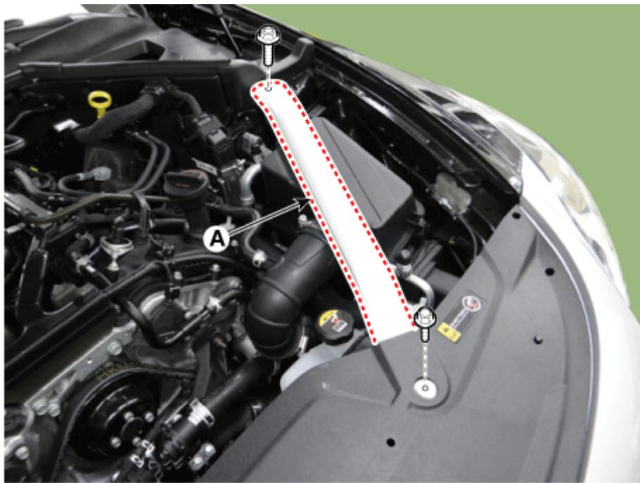
3. Remove the reservoir tank (A).
